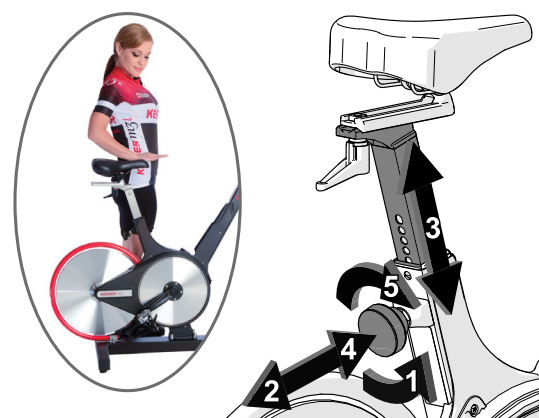
Figure 9. Seat Height Adjustment
