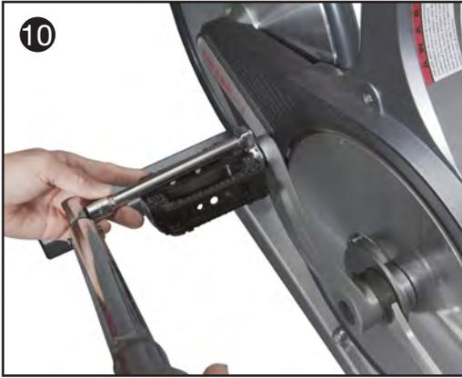
**Step 2:** With a clean cloth, wipe the threaded area of the pedals. Apply Loctite 242 to the pedal threads. Install the pedals into the crank arms, use the 15mm open-end wrench to tighten. Finish with the torque wrench, 15mm crowfoot, and 6" extension. Torque pedals to 47 Nm (35 ft-lbs) (Fig. 10).
