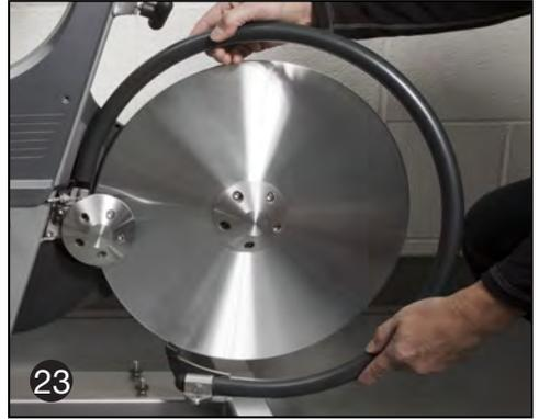
**Step 5:** Swing the tube over the flywheel, aligning the tube centered with the flywheel.
