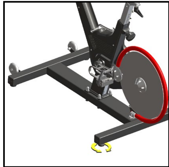
Figure 25. Leveler Foot Adjustment
